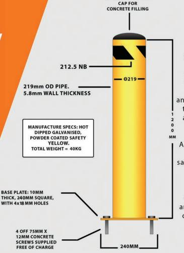
All our bollards are hot dipped galvanised after manufacture to prevent rusting. Custom powder coating colours and custom safety tape options are available, talk to us about your requirements. All stock lines are powder coated safety yellow with a black & clear chevron sticker around the top. Concrete fixings are supplied with our bollards free of charge.
