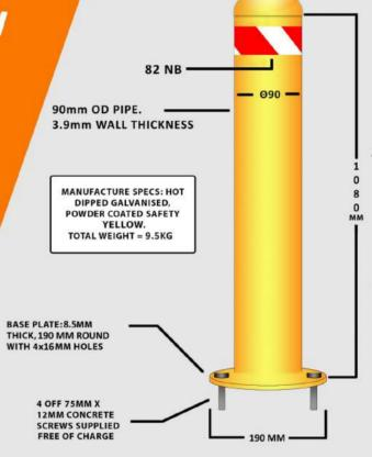
All our bollards are hot dipped galvanised after manufacture to prevent rusting. Custom powder coating colours and custom safety tape options are available, talk to us about your requirements. All stock lines are powder coated safety yellow with a black & clear chevron sticker around the top. Concrete fixings are supplied with our bollards free of charge.
