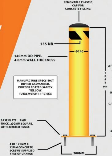
All our bollards are hot dipped galvanised after manufacture to prevent rusting. Custom powder coating colours and custom safety tape options are available, talk to us about your requirements. All stock lines are powder coated safety yellow with a black & clear chevron sticker around the top. Concrete fixings are supplied with our bollards free of charge.
